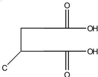
Metallic salt formation can be initiated between the carboxylic functionality and iron ions on the surface of a steel surface for example.
