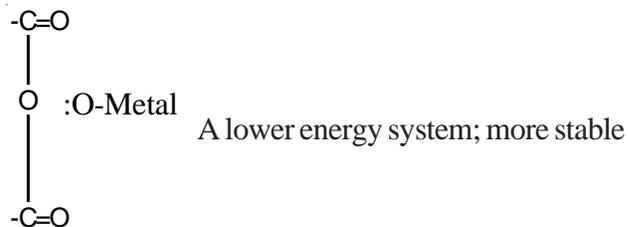
In the case of a metal where the oxide is tightly bound to the metal (for example in the case of aluminum) this bond can be very effective. If the oxide easily flakes away from the metal (as in the case of zinc for example), the PBD-MA is effective in interacting with the oxide film but the film itself is easily shed and overall bonding is not as effective.
