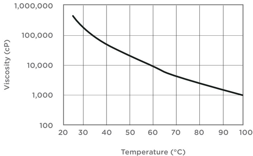
Figure 1: Ricon 100 viscosity vs. temperature.
