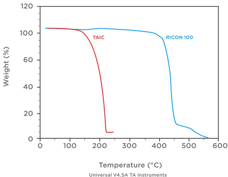
**Figure 3:** TGA in oxygen (10 °C/min) of neat Ricon 100 and TAIC.
