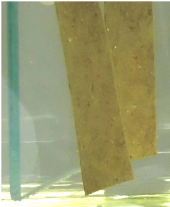
Figure 1: Photo of brown paper strips quickly coming off a glass plate in less than one minute after immersion into an 80 °C caustic solution.
