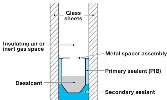
Figure 1: Schema of an insulated glass unit (IGU).
