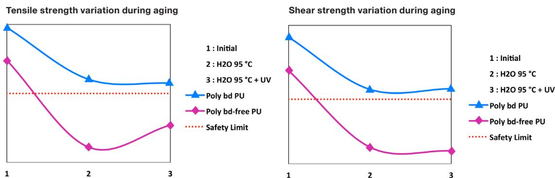
**Figure 6:** Comparison of PU properties: Poly bd-based vs. Poly bd-free PU. A Poly bd-based PU sealant will retain tensile and shear strength after aging.
