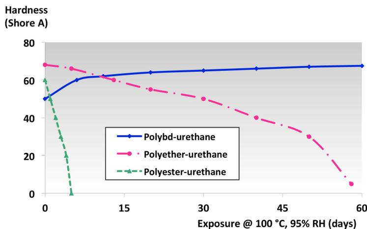
**Figure 7:** Comparative hydrolytic stability of polyurethanes based on various polyols.<sup>3</sup> A Poly bd-based PU sealant will retain original properties over time.
