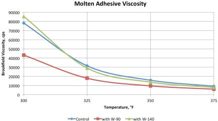
As little as 2 weight percent of Cleartack W-90 can dramatically reduce the molten viscosity of an SBC-based hot melt adhesive, especially at low temperatures. This can dramatically improve the ability to coat or spray the adhesive, reducing defects and improving performance.
