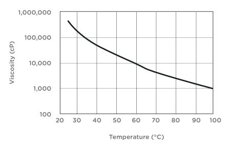
Figure 1: Ricon 100 viscosity vs. temperature.
