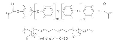
Figure 1: Structures of vinyl functional polyphenylene ether resin (left) and Ricon 100 (right).
