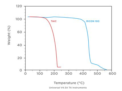
Figure 3: TGA in oxygen (10 °C/min) of neat Ricon 100 and TAIC.
