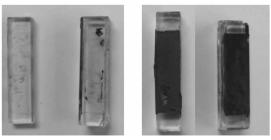
Figure 8: Comparative adhesion to glass after UV exposure of Poly bd-free (left) and Poly bd-based (right) PUs. Only the Poly bd-based PUs maintain good adhesion to glass after UV aging.
