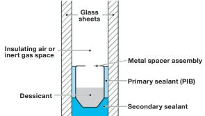
Figure 1: Schema of an insulated glass unit (IGU).
