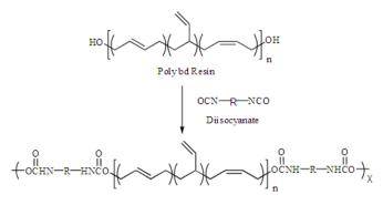
Figure 2: Poly bd-based polyurethane.
