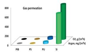
Figure 4: Gas permeation rates for polyisobutyl (PIB), polysulfide (PS), polyurethane (PU) and silicone (Si) sealants.
